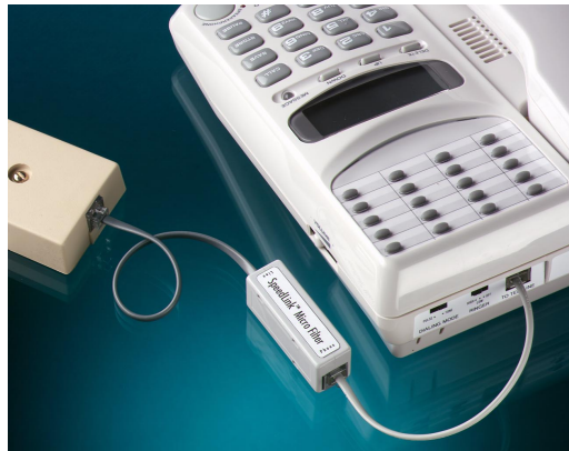
Figure 7: In-Line Microfilter Installation
